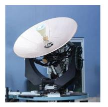
Satcom systems developer EM Solutions sought a lighter, simpler-to-install design for the identical azimuth arms on its King Cobra naval-mounted satellite. Partner ACS Australia provided a design and manufacturing solution that resulted in a 65% lighter arm versus metal, reducing dozens of pieces to one per arm. Source | EM Solutions via ACS Australia
