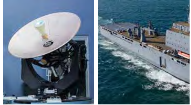
EM Solutions King Cobra satcom with composite azimuth arms (left); and installed and commissioned satcom on a sailing navy vessel (right).
