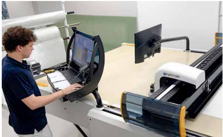
Pathfinder automated composite material ply-cutting machine.
