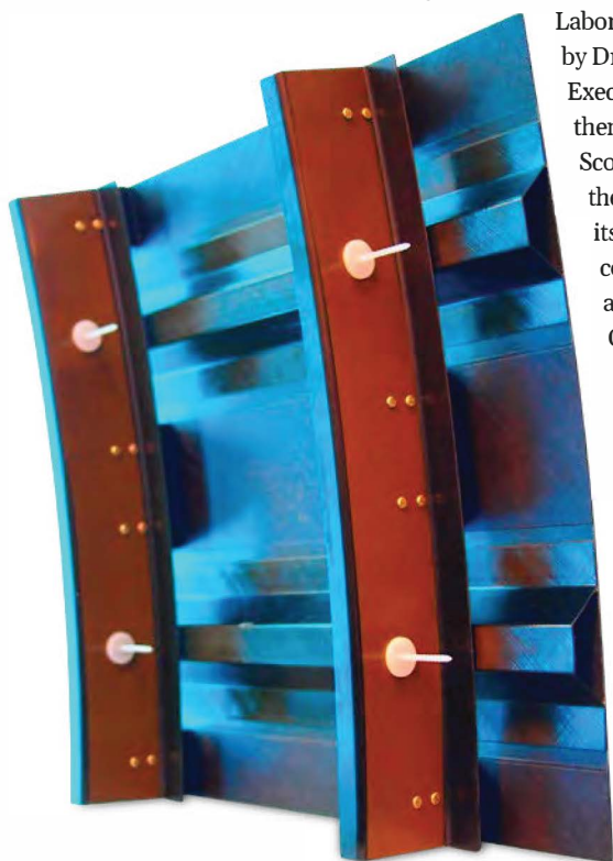
Composite Fitting Attachment (COFA) demonstrator – thermoplastic bracket ultrasonically welded to thermoset panel, developed by ACS Australia.
